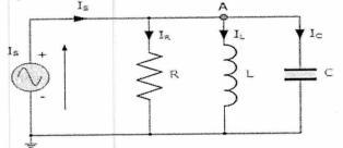
Assume the input current as  $I_s(t) = I_m \sin(\omega t)$  and the output as voltage v(t) across the capacitor.
